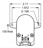
This option includes molded ears on the **E5** base which enable it to be mounted to a 1.812" diameter bolt circle. The mounting holes are designed to fit 4-40 screws. Because the ears are molded to the **E5** base this does not increase the thickness of the encoder and does not add to the required shaft length. This option will work with shaft lengths of .445" to .570"
