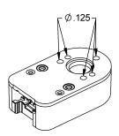
The **3**-option makes all five of these hole diameters .125". The .438" diameter center hole can also mate with a motor boss.
