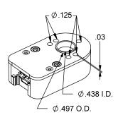
The **A**-option adds a .497" diameter alignment shoulder designed to slip into a .500" diameter recess in the mounting surface centered around the shaft.
